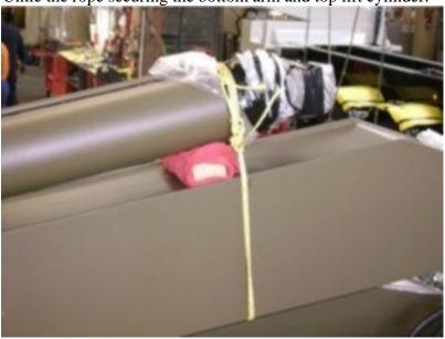
2. Remove the packaging protecting the end of the top arm and securing the sensor cabling.
